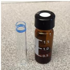
Figure 1. An HPLC vial loaded with sample (right) and an optional 400  $\mu\text{L}$  glass insert (left).
